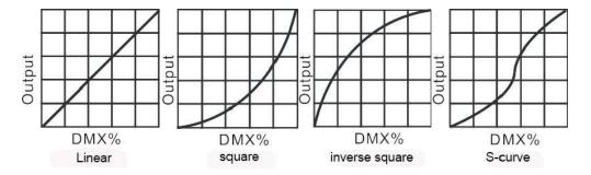
Mode 1 (linear): With the increase of DMX value, the increase of light intensity tends to be linear:
