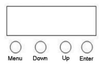
The LCD system includes Menu, Down, Up, and Enter buttons. Press "Menu" to enter the menu or to go back from a sub-menu. Use "Up"/"Down" to navigate through the choices, and use "Enter" to save your choices. *Note, the options below are numbered, and the "Up" key brings you forward in number, which is down on the screen.*
