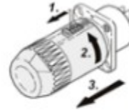
discharge the power cable
