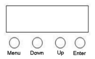
The LCD system includes Menu, Down, Up, and Enter buttons. Press "Menu" to enter the menu or to go back from a sub-menu. Use "Up"/"Down" to navigate through the choices, and use "Enter" to save your choices.
