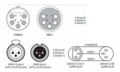
For installations where the DMX cable has to run a long distance or is in an electrically noisy environment, it is recommended to use a DMX terminator. This helps in preventing corruption of the digital control signal by electrical noise and reflections. The DMX terminator is simply an XLR plug with a 120  $\Omega$  resistor connected between pins 2 and 3, which is then plugged into the output XLR socket of the last fixture in the chain. Please see illustrations below:
