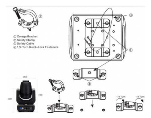
Regardless of the rigging option you choose for your TX6 Beam, always be sure to secure your fixture with a safety cable. The fixture providers a built-in rigging point for a safety cable on the hanging bracket as illustrated above. Be sure to only use the designated rigging point for the safety cable and never secure a safety cable to a carrying handle.
