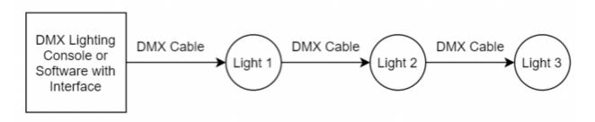
DMX Cables can be 3-pin or 5-pin. These use the same type of data, and in the 5-pin only pins 1, 2, and 3 are used. The cable should be a 2 conductor, shielded cable of at least 110 ohms resistance. Microphone cable is not DMX cable.
